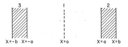
Fig. D.1. Three-slab heat flow geometry.
